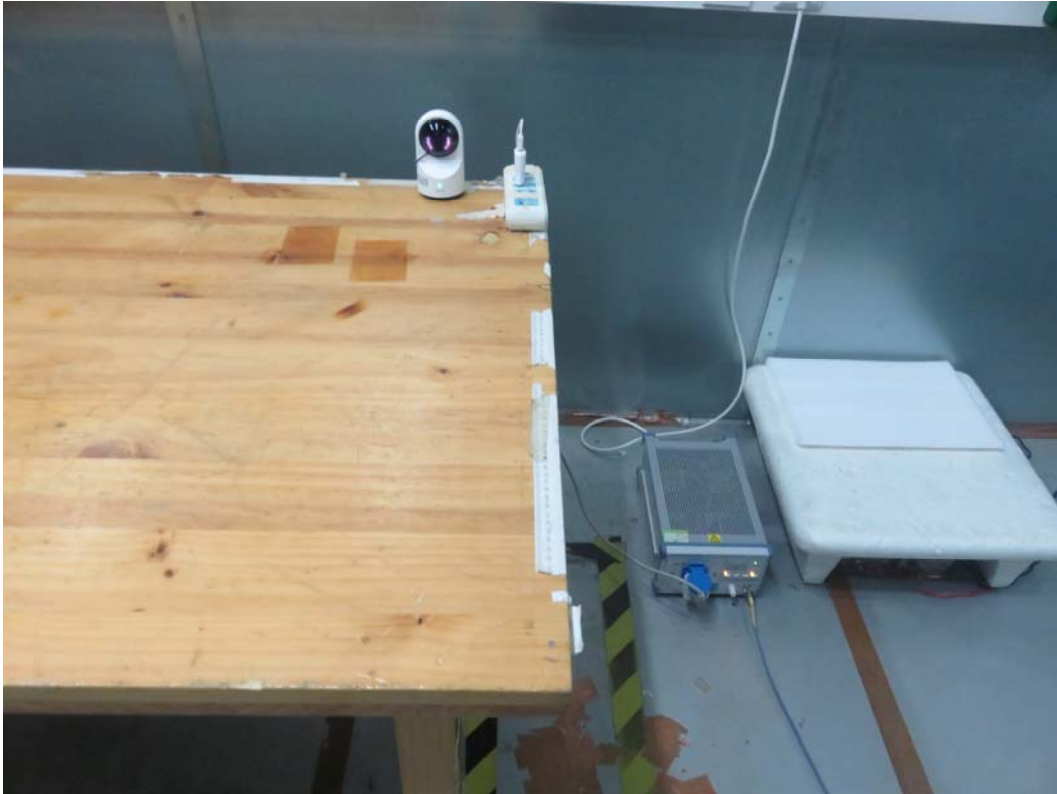
Picture 3 Conducted Emission Test Setup
