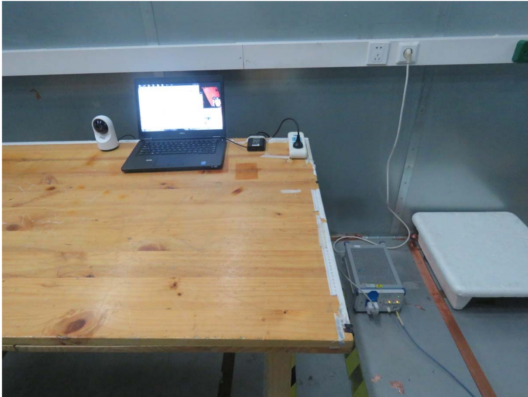
Picture 3 Conducted Emission Test Setup
