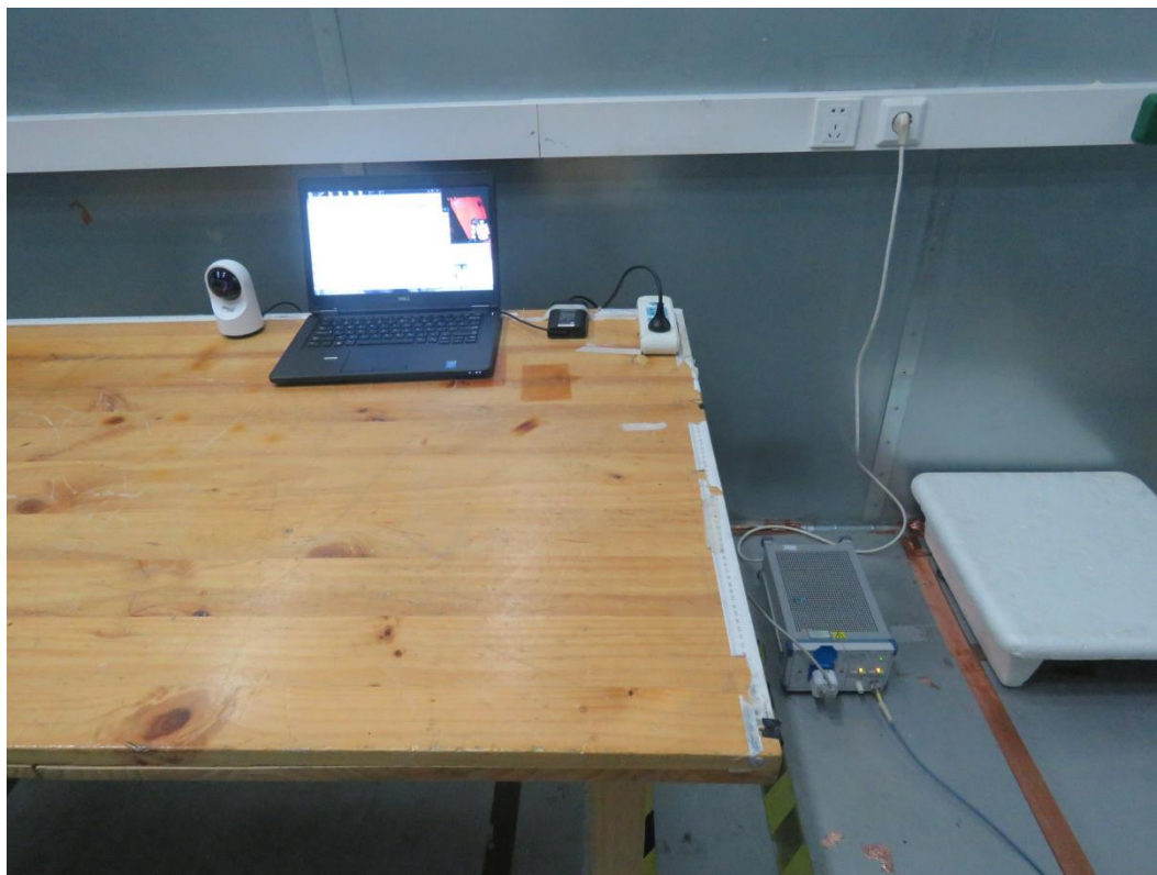
Picture 3 Conducted Emission Test Setup
