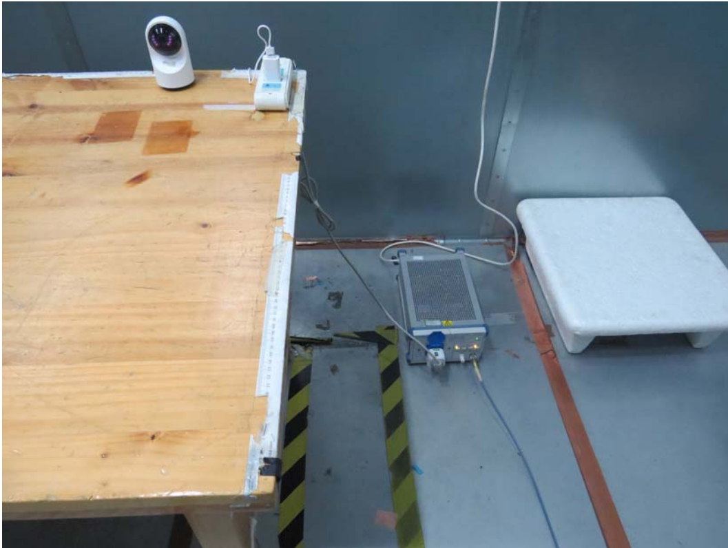
Picture 3 Conducted Emission Test Setup
