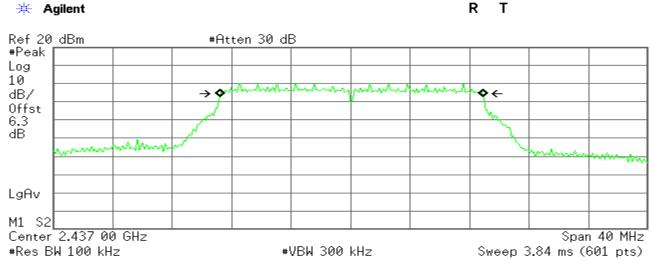
Occupied Bandwidth 17.7471 MHz Occ BW % Pwr 99.00 % x dB -6.00 dB
