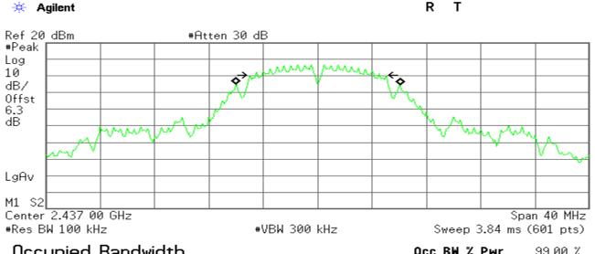
Occupied Bandwidth 12.0304 MHz Occ BW % Pwr 99.00 % x dB -6.00 dB
