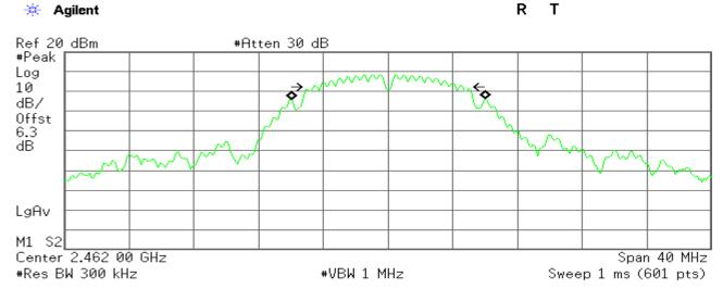
Occupied Bandwidth 11.9832 MHz Occ BW % Pwr 99.00 % x dB -6.00 dB
