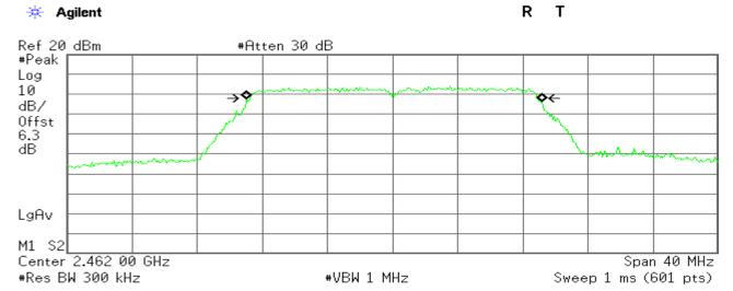
Occupied Bandwidth 18.1562 MHz 0cc BW % Pwr 99.00 % x dB -6.00 dB
