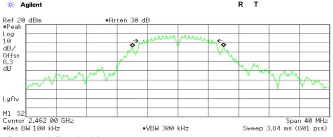
Occupied Bandwidth 11.9971 MHz Occ BW % Pwr 99.00 % x dB -6.00 dB
