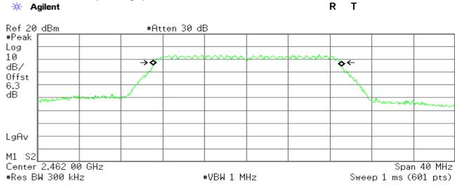
Occupied Bandwidth 18.0481 MHz Occ BW % Pwr 99.00 % + dB -6.00 dB
