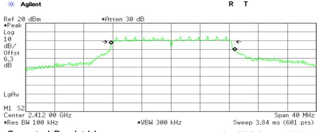
Occupied Bandwidth 17.0724 MHz Occ BW % Pwr 99.00 % x dB -6.00 dB
