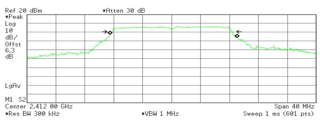
Occupied Bandwidth 17.6008 MHz Occ BW % Pwr 99.00 % -6.00 dB x dB
