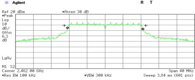
Occupied Bandwidth 16.8525 MHz Occ BW % Pwr 99.00 % x dB -6.00 dB
