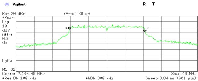
Occupied Bandwidth 16.6608 MHz Occ BW % Pwr 99.00 % x dB -6.00 dB
