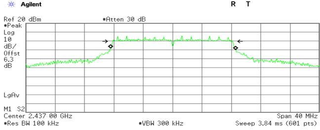
Occupied Bandwidth 17.1124 MHz 0cc BW % Pwr 99.00 % x dB -6.00 dB
