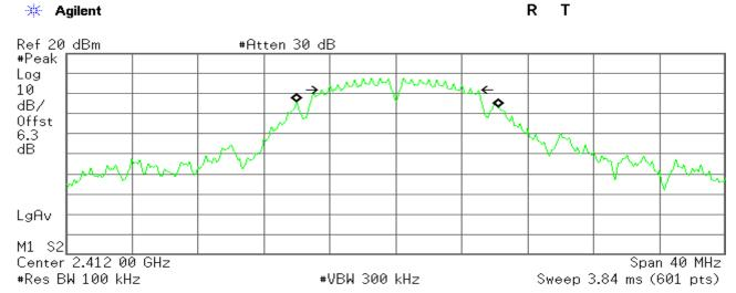
Occupied Bandwidth 12.1513 MHz Occ BW % Pwr 99.00 % x dB -6.00 dB
