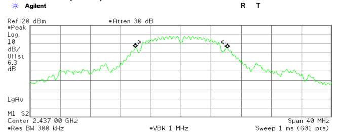
Occupied Bandwidth 12.1645 MHz 0cc BW % Pwr 99.00 % x dB -6.00 dB
