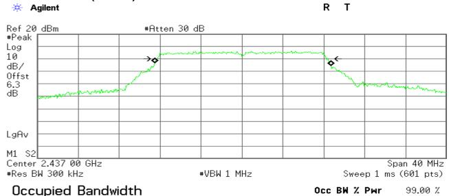
Transmit Freq Error 112.776 kHz x dB Bandwidth 16.714 MHz
