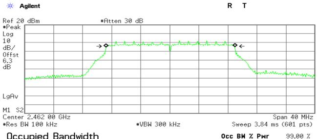
Occupied Bandwidth 17.7665 MHz Occ BW % Pwr 99.00 % x dB -6.00 dB
