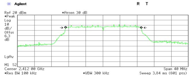
Occupied Bandwidth 17.7739 MHz Occ BW % Pwr 99.00 % x dB -6.00 dB
