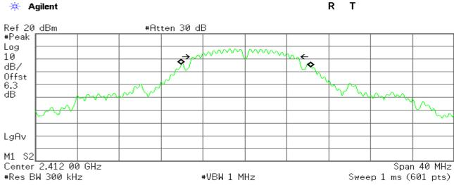
Occupied Bandwidth 12.3629 MHz Occ BW % Pwr 99.00 % x dB -6.00 dB
