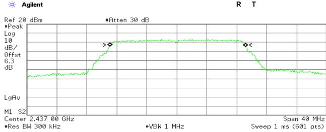
Occupied Bandwidth 18.1751 MHz Occ BW % Pwr 99.00 % × dB -6.00 dB
