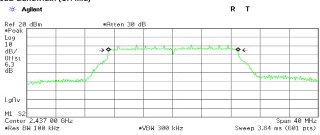
Occupied Bandwidth 17.7643 MHz Occ BW % Pwr 99.00 % x dB -6.00 dB
