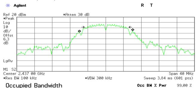
Transmit Freq Error 67.776 kHz x dB Bandwidth 8.632 MHz
