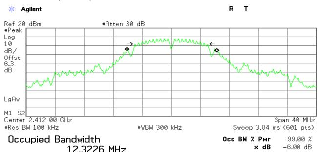
Transmit Freq Error 84.980 kHz x dB Bandwidth 9.163 MHz
