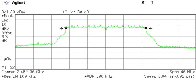
Occupied Bandwidth 17.7302 MHz Occ BW % Pwr 99.00 % x dB -6.00 dB
