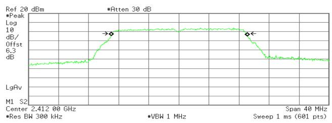
Occupied Bandwidth 18.1686 MHz Occ BW % Pwr 99.00 % × dB -6.00 dB
