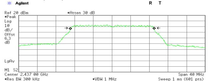
Occupied Bandwidth 17.9740 MHz Occ BW % Pwr 99.00 % x dB -6.00 dB
