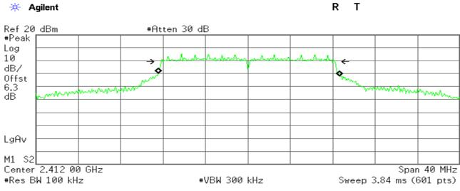
Occupied Bandwidth 17.1504 MHz Occ BW % Pwr 99.00 % -6.00 dB x dB
