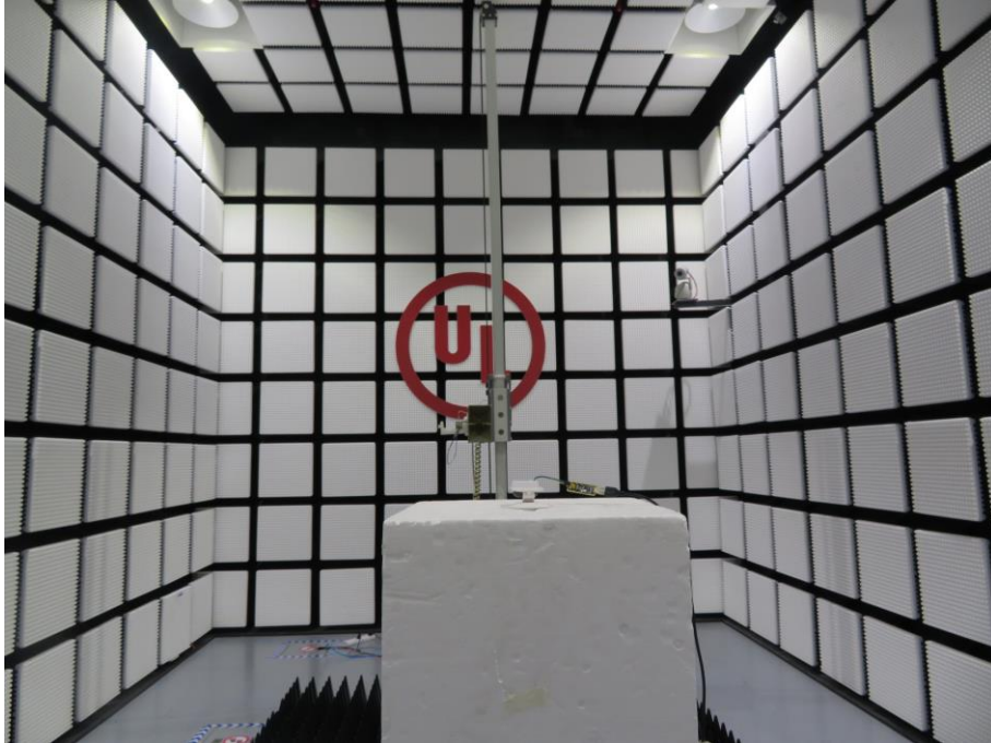
RADIATED RF MEASUREMENT SETUP (ABOVE 1 GHz)
