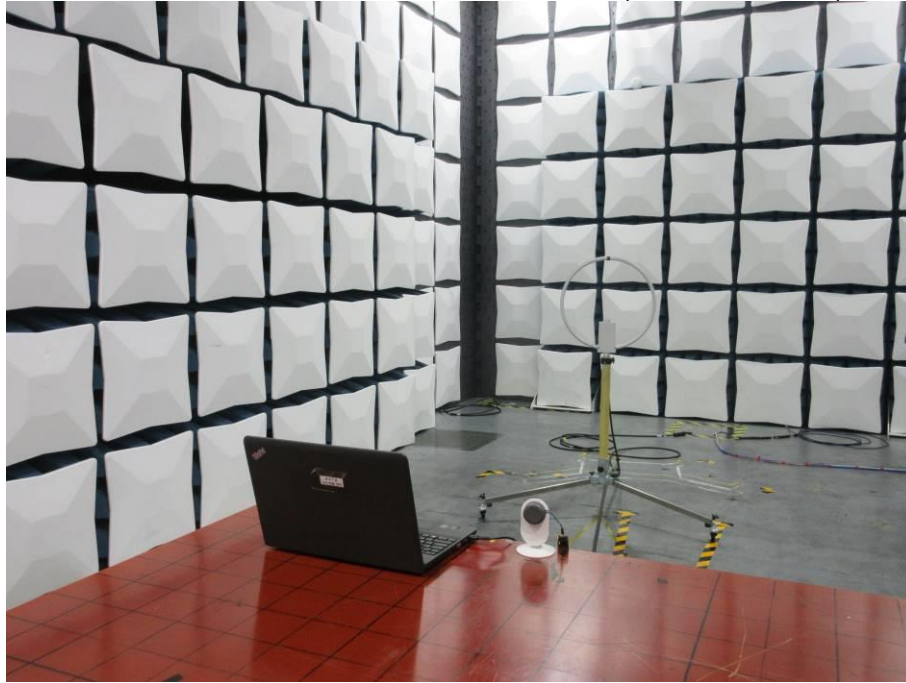
RADIATED RF MEASUREMENT SETUP (9KHz ~ 30 MHz)
