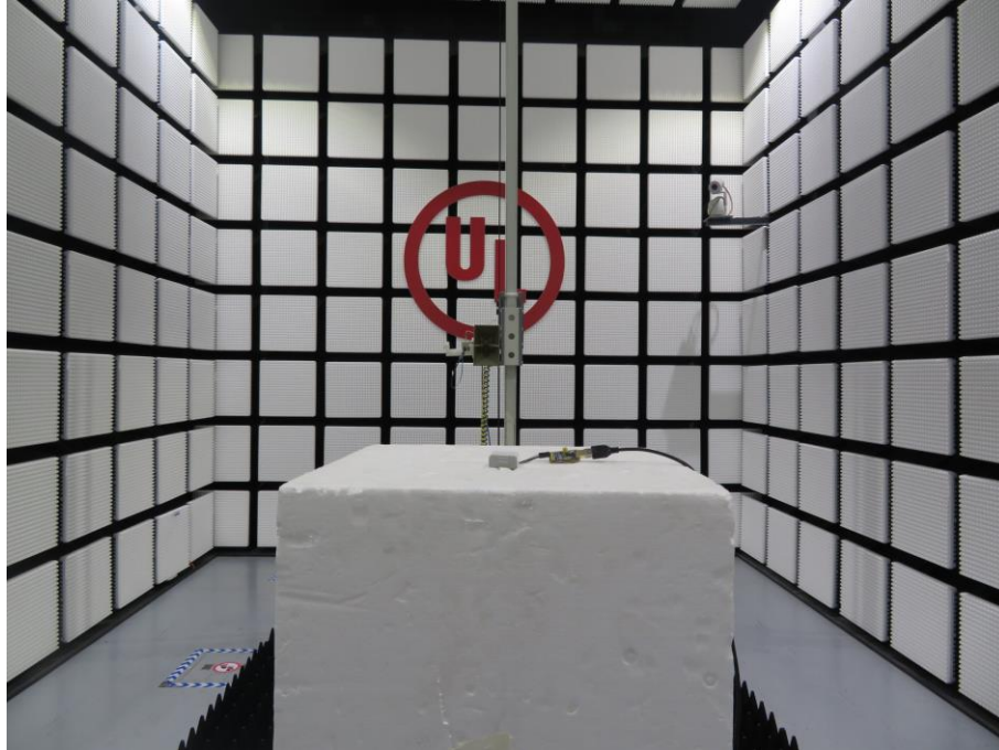
RADIATED RF MEASUREMENT SETUP (ABOVE 1 GHz)
