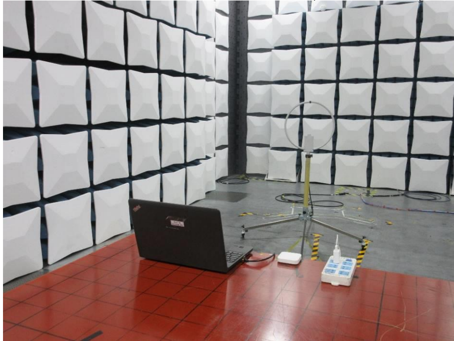
RADIATED RF MEASUREMENT SETUP (9KHz ~ 30 MHz)
