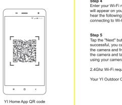
Enter your Wi-Fi network password and tap the "Please choose Wi-Fi" buttonA QR code will appear on your phone's screen. Point theQR code towards the camera lens until you hear the following messages 'QR code scan is successful, connecting to Wi-Fi" and "Wi-Fi is connected". Step 5
