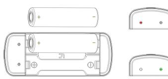
Red indicator normally on: The battery voltage is lower than 4.2V
