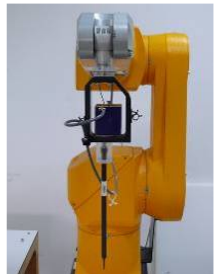
Figure 3. EX3DV4 E-field probe
