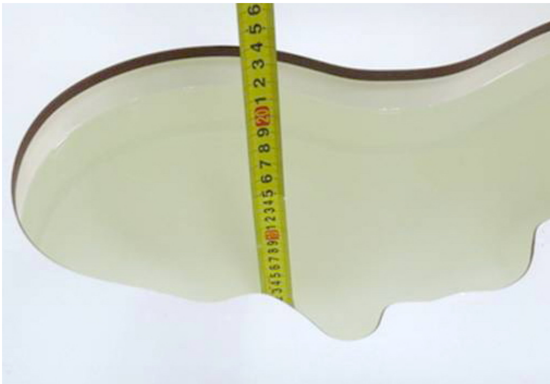
Picture 3: Liquid depth in the head Phantom (2450 MHz, 15.4cm depth)
