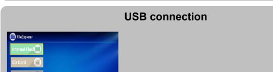
• Connect USB line interface, plug in the machine of right side USB interface, the other point is inserted in the computer USB interface connection, drag down the status bar, and then show USB connection status, that will be appear "USB connection", prompting USB connection.
