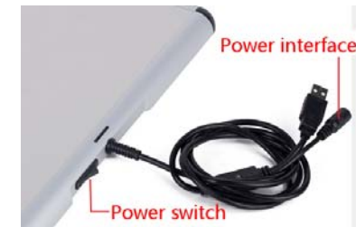
Power switch and interface
