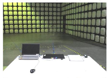
1.4 Radiated Emissions(30MHz-1GHz) Test Setup
