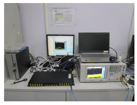
1.3 Emission Mask & Radiated Emissions(9kHz-30MHz) Test Setup
