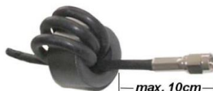
Figure 3 Antenna cable with EMC loop antenna
