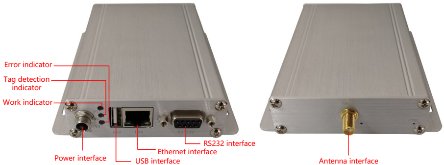
Figure 1 Description of reader appearance and hardware interfaces
