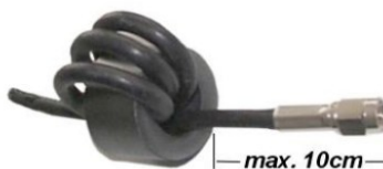
Figure 3 Antenna cable with EMC ring core
