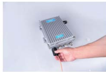
6, The LORA feeder connected to the LORA interface, after installation, the FRP antenna on the heat shrinkable tube heating, and then wrapped with high temperature adhesive
