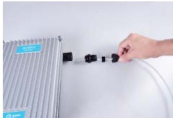
8, Insert the cable into the RJ45 hole as shown
