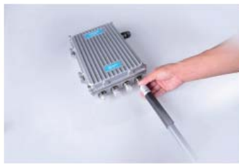
5, Insert the FRP antenna into the 4G/WIFI/GPS interface and check whether the connection is tightened
