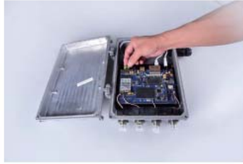
2, After opening, insert the prepared SIM data traffic card, as shown in Figure
