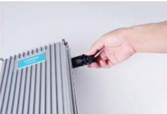
7, As shown, unscrew the RJ45 waterproof head
