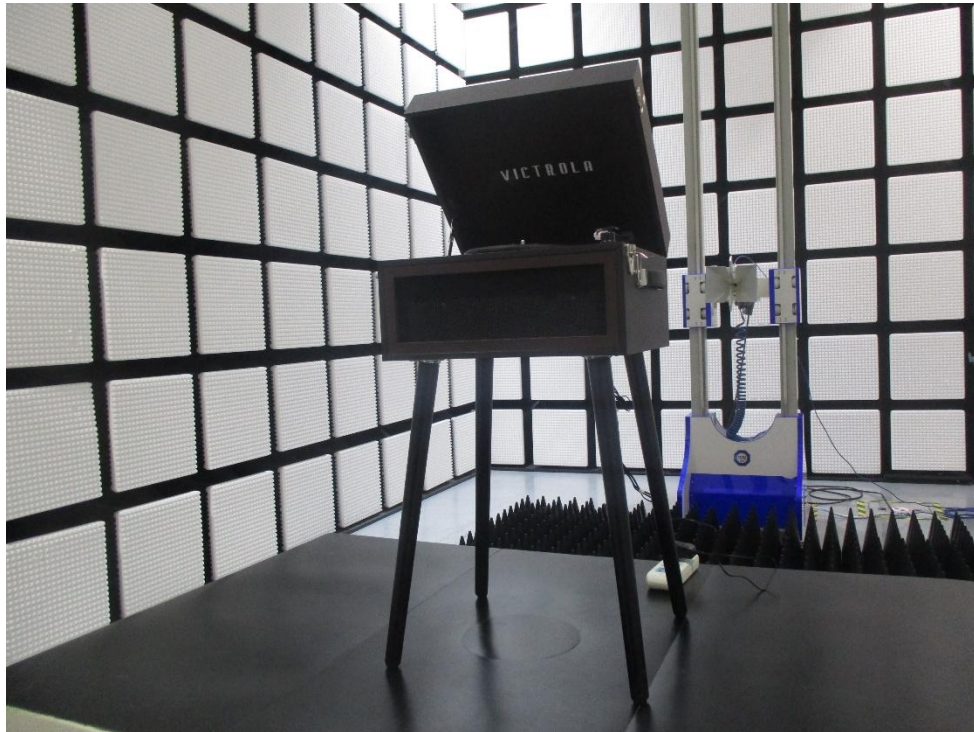
Radiated Emission Test above 1GHz
