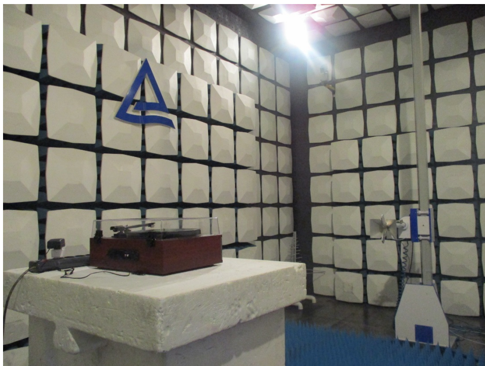
Photograph 3: Set-up for Radiated Spurious Emission, 1GHz - 18GHz
