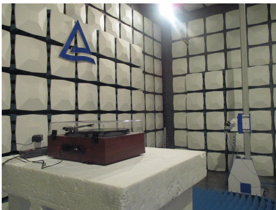
Photograph 4: Set-up for Radiated Spurious Emission, 18GHz - 26.5GHz
