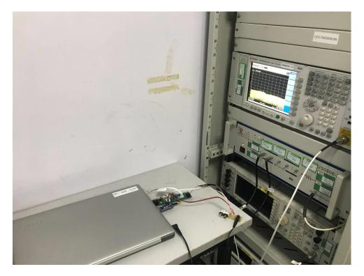
Conducted Emissions at AC Power Line (150kHz-30MHz)
