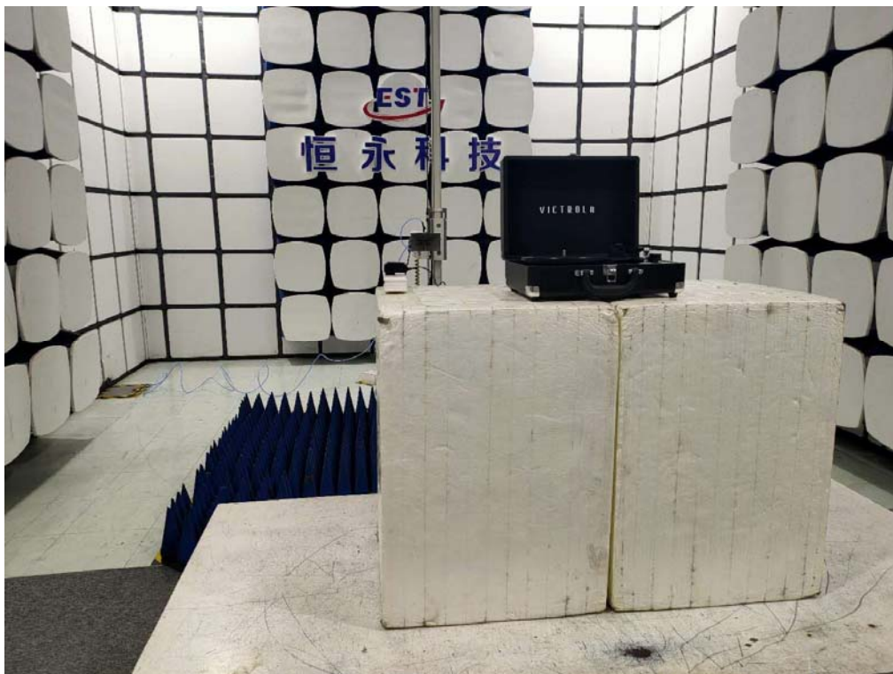
Radiated Test (Above 1GHz)
