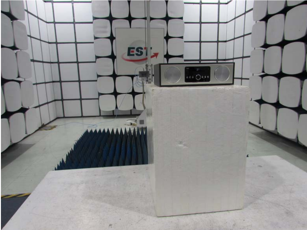
Radiated Test (1000-25000 MHz)
