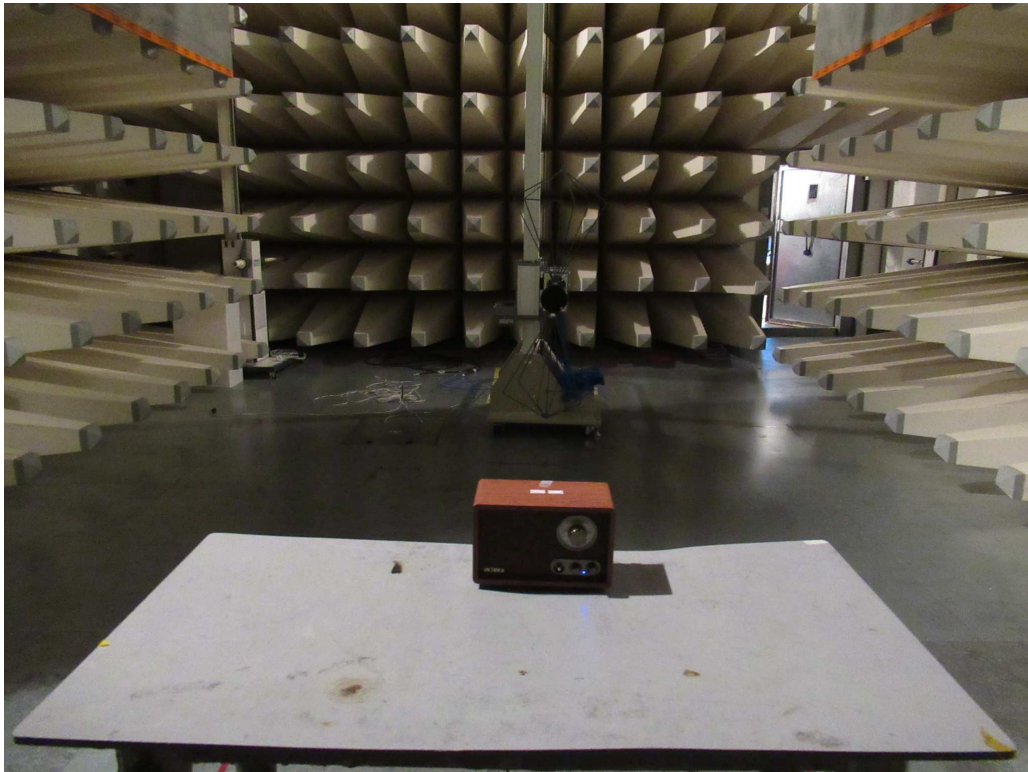
Set-up for Radiated Emission
