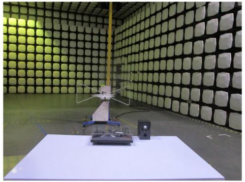
Radiated Spurious Emissions (Above 1GHz) & Radiated Emissions which fall in the restricted bands
