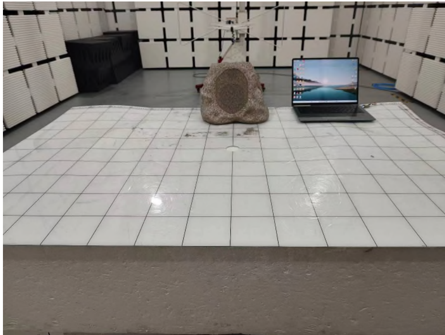
Photograph 1: Set-up for Radiated Spurious Emission, 30MHz - 1GHz
