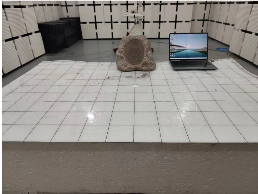
Photograph 1: Set-up for Radiated Spurious Emission, 30MHz - 1GHz
