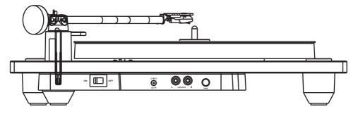
Method 2: Insert the AC/DC Adapter plug into the DC Cable Splitter, plug one end of DC Cable Splitter into the DC IN Jack of the Turntable, then plug another end of the AC/DC Adapter into the AC Walloutlet.
