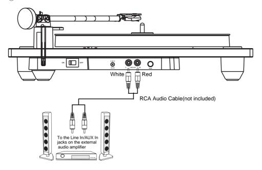
(2) Connect the Turntable through LINE OUT Jacks to the LINE IN jack of the speaker
