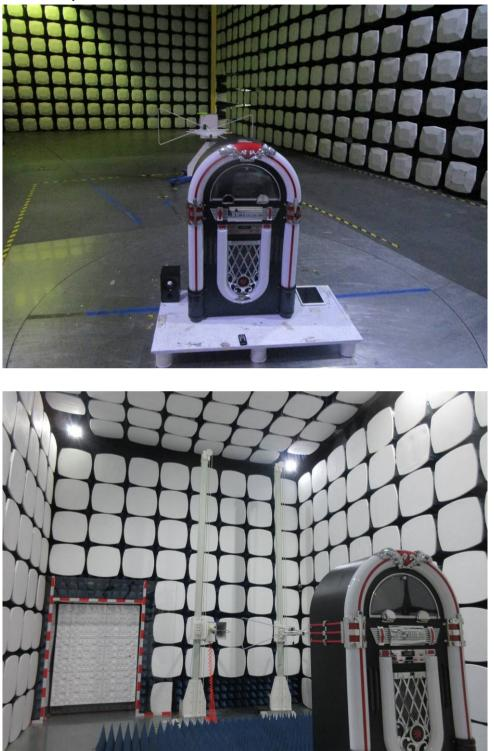
Remark: The transmitter part of the EUT was kept on the high 1.5m above 1GHz according to the lifting platform during the test.
