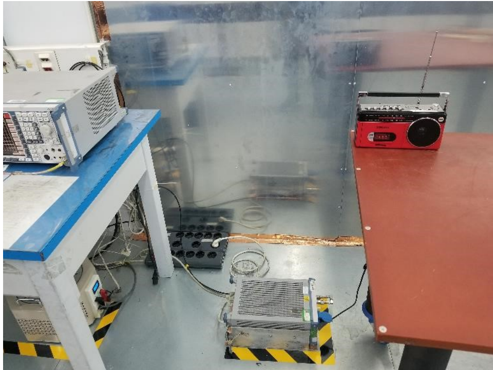
Photograph 5: Set-up for Conducted Emission on AC Mains
