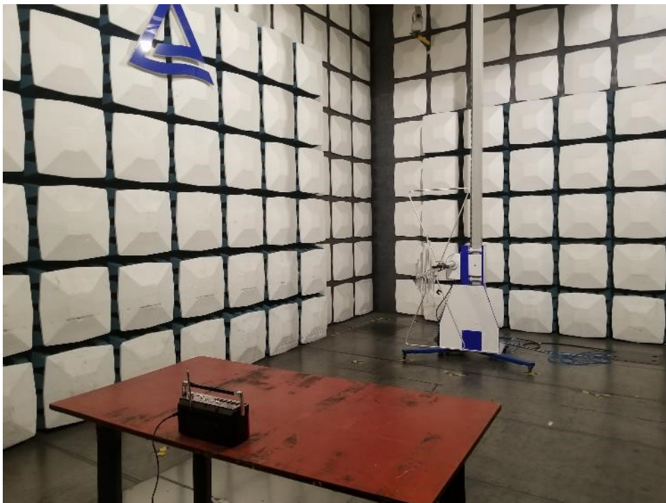
Photograph 2: Set-up for Radiated Spurious Emission, 30MHz - 1GHz
