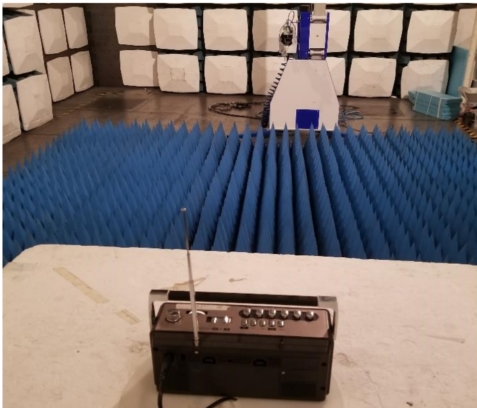
Photograph 4: Set-up for Radiated Spurious Emission, 18GHz - 26.5GHz
