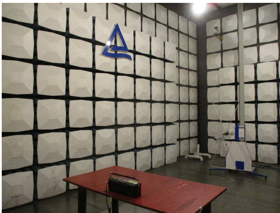
Photograph 2: Set-up for Radiated Spurious Emission, 30MHz - 1GHz
