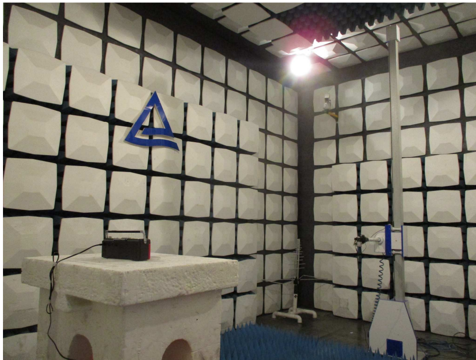
Photograph 4: Set-up for Radiated Spurious Emission, 18GHz - 26.5GHz
