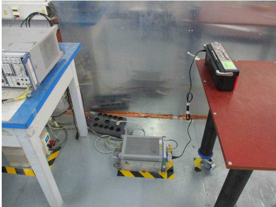
Photograph 5: Set-up for Conducted Emission on AC Mains
