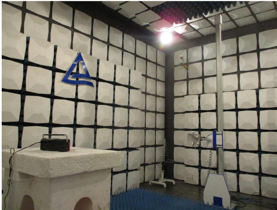
Photograph 4: Set-up for Radiated Spurious Emission, 18GHz - 26.5GHz
