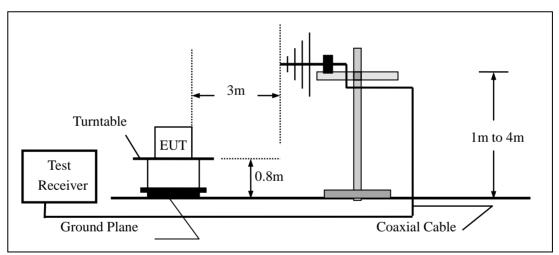
(c) For radiated emissions above 1000MHz
