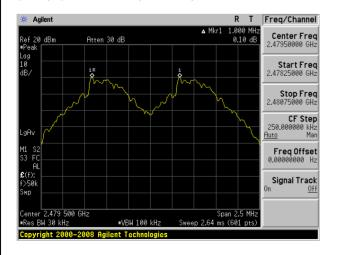
(2Mbps) Channel Separation plot on channel 77-78
