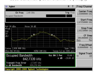
20dB Bandwidth plot on channel 78 (2Mbps)
