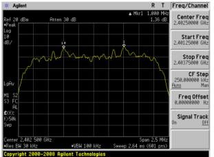
(1Mbps) Channel Separation plot on channel 39-40
