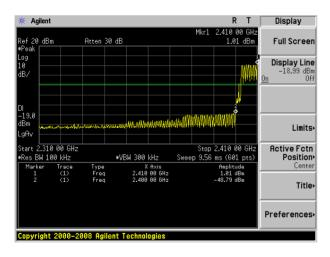
GFSK: Band Edge-High Channel (Hopping Mode)
