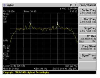
(1Mbps) Channel Separation plot on channel 77-78
