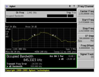
20dB Bandwidth plot on channel 39 (2Mbps)
