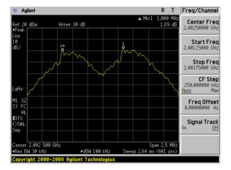
(2Mbps) Channel Separation plot on channel 00-01
