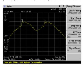
(2Mbps) Channel Separation plot on channel 39-40
