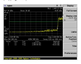
$\pi$  /4-DQPSK: Band Edge-High Channel (Hopping Mode)
