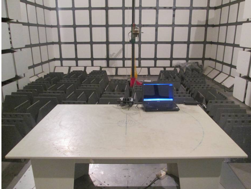
Radiated Emissions Front View (Above 1GHz)
