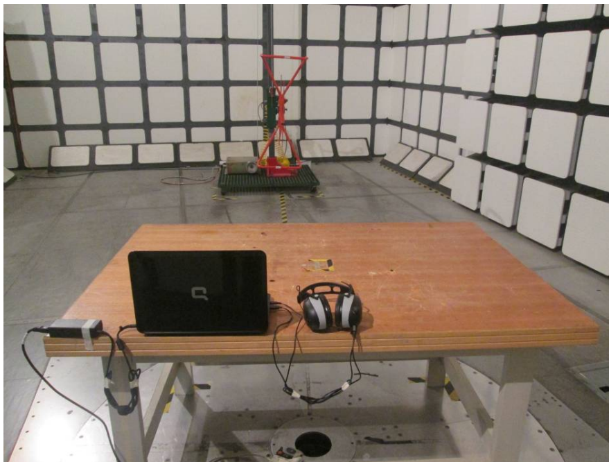
Radiated Emissions Rear View (Below 1GHz)
