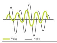
Clear Voice Tracking seeks voices in background/ environmental noise and reduces the noise to improve speech intelligibility. The user can select standard microphone filtering by turning off the Surround Sound Filtering in the setup menu. The default setting is Surround Sound Filtering ON.
