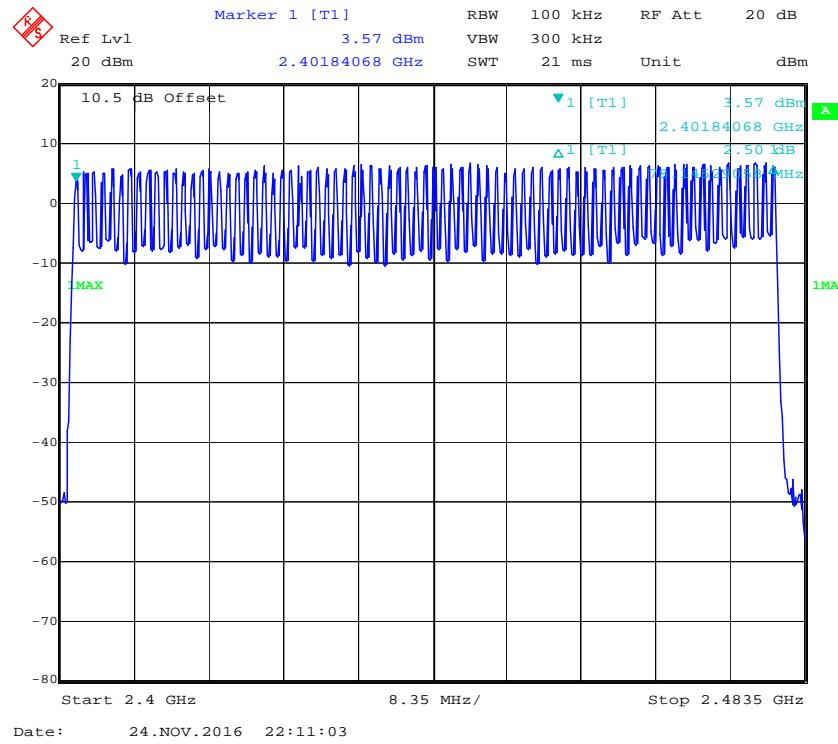
**EDR ( $\pi/4$ -DQPSK): Number of Hopping Channels**
