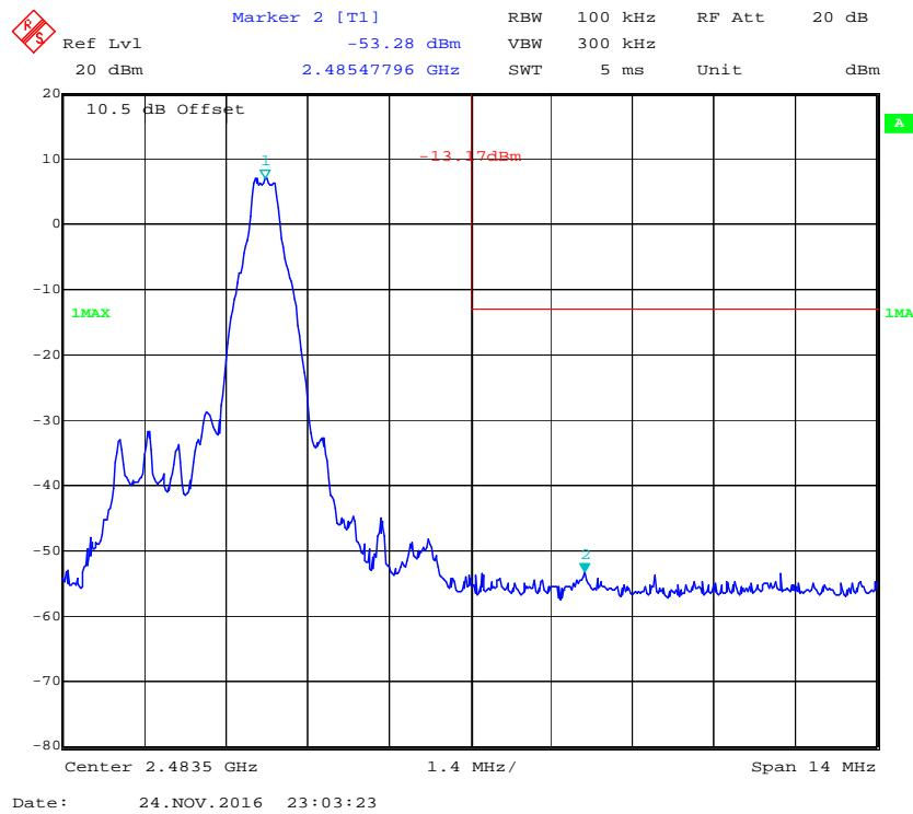
**EDR ( $\pi/4$ -DQPSK): Band Edge-Left Side**
