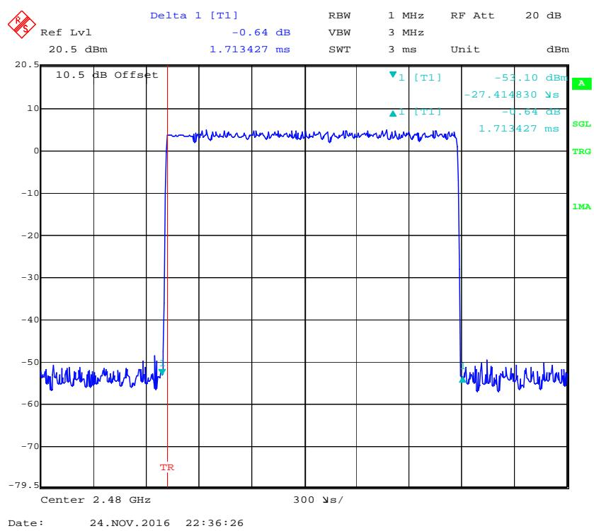
**Pulse time, Low Channel, 3DH5**
