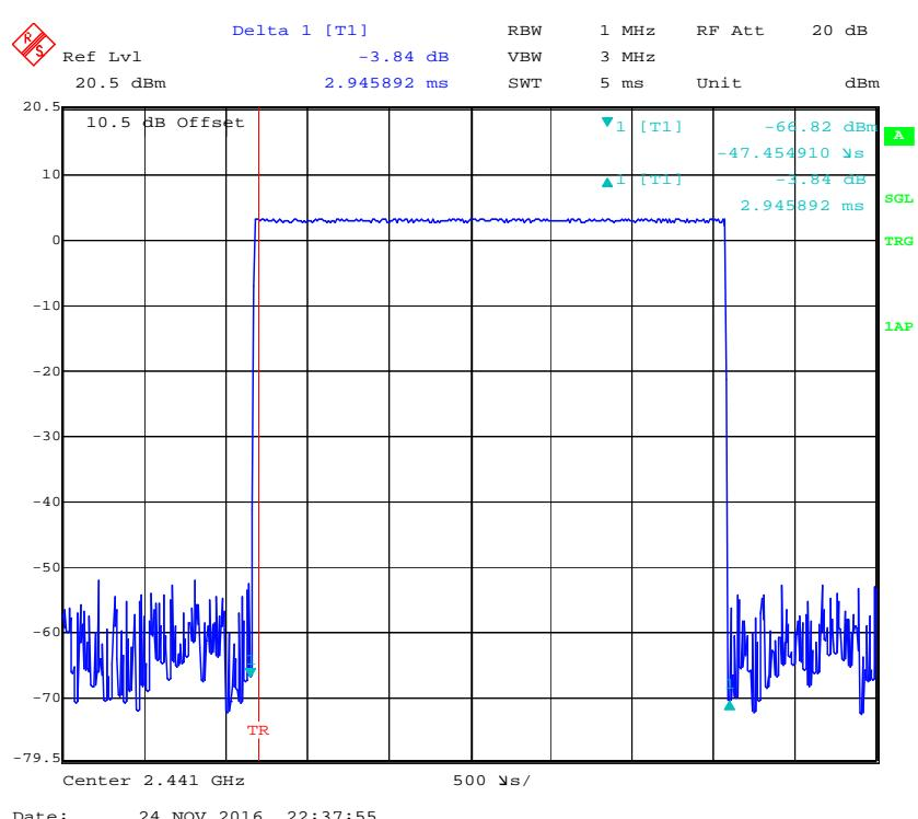
**Pulse time, High Channel, DH5**
