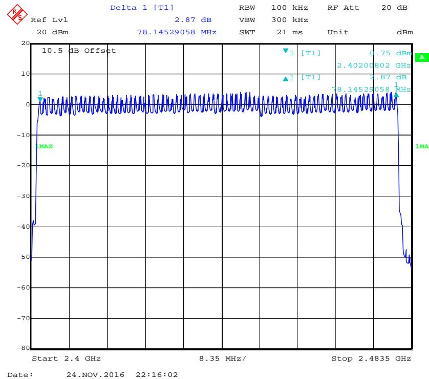
**EDR (8DPSK): Number of Hopping Channels**
