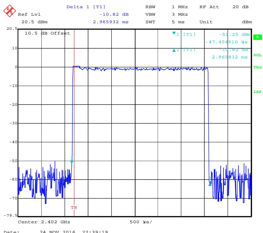
**Pulse time, Middle Channel, 2DH5**
