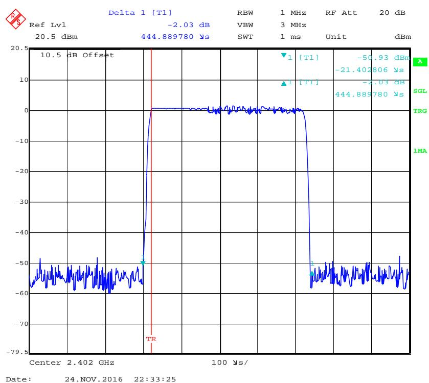
**Pulse time, Middle Channel, 2DH1**
