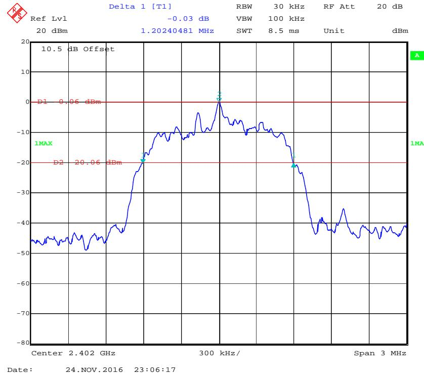
**EDR ( $\pi/4$ -DQPSK): Middle Channel**
