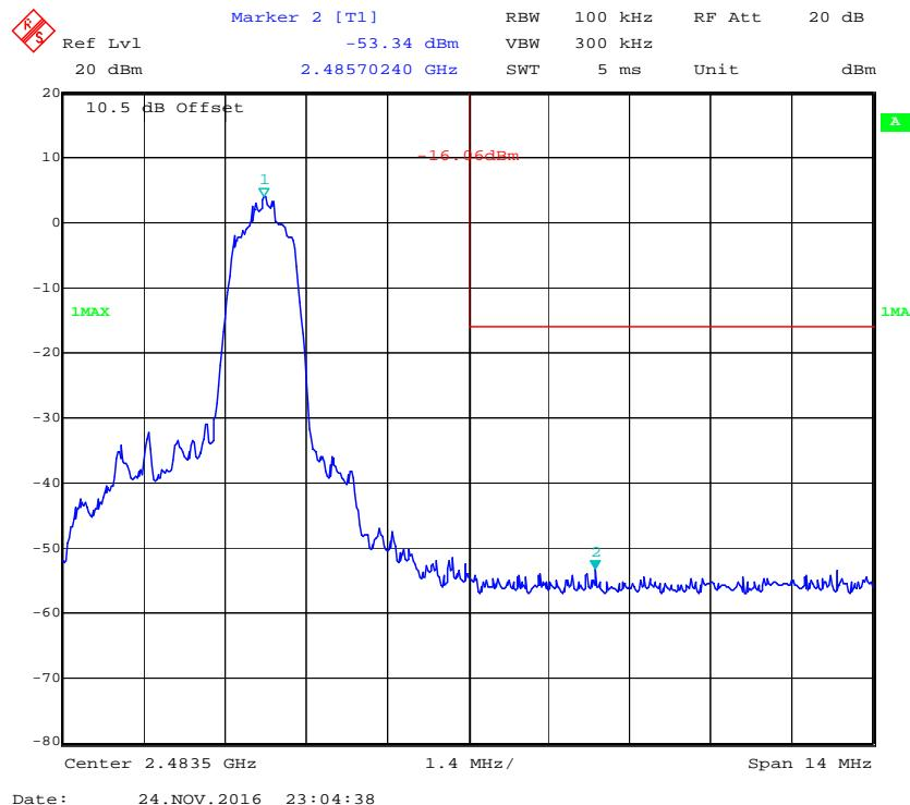
**EDR (8DPSK): Band Edge-Left Side**
