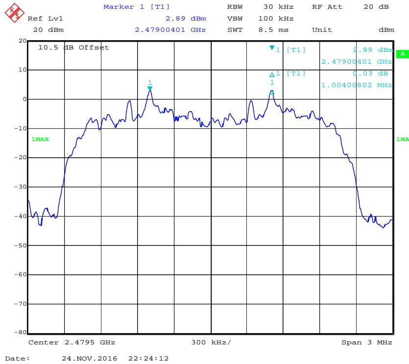
**EDR (8DPSK): Low Channel**
