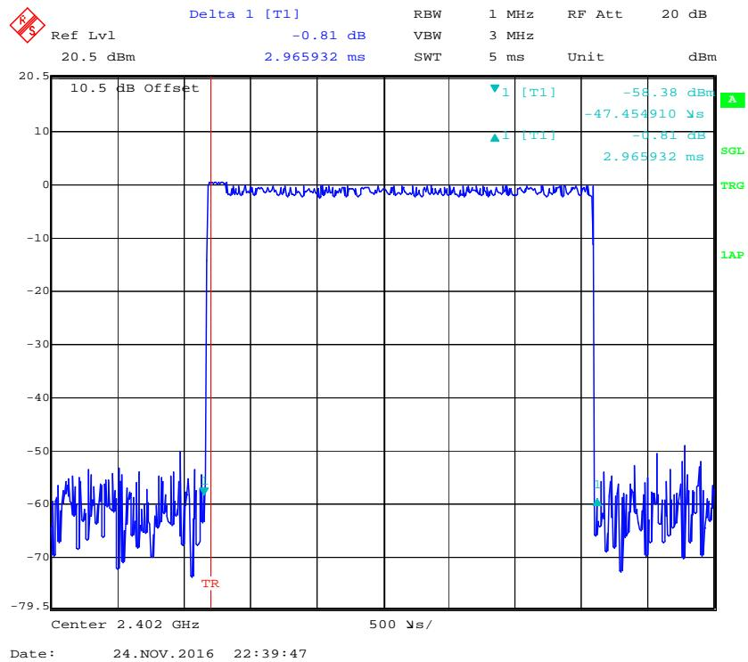
**Pulse time, Middle Channel, 3DH5**
