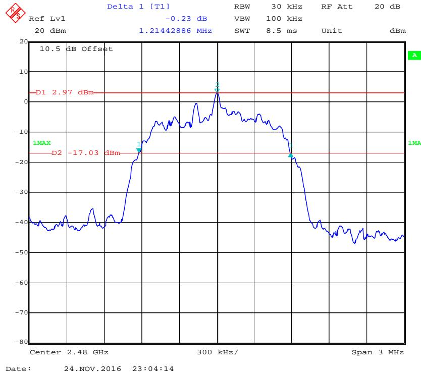
**EDR (8DPSK): Low Channel**
