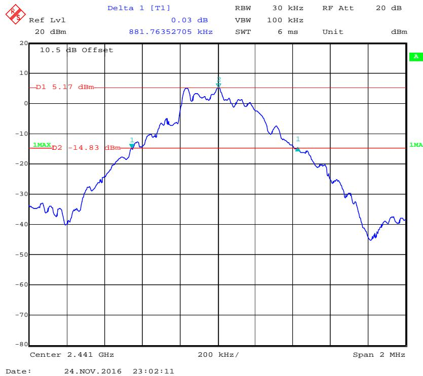
**BDR (GFSK): High Channel**
