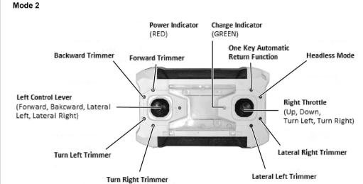
Push the Right Throttle up or down, the Quadcopter flies upward or downward.
