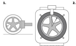
Break the bead of the tire ensuring the valve is located on Place the valve through the valve hole, ensuring the rubber When the tire is dismounted the valve must be located at 1 o'clock to the tire fitting head.
