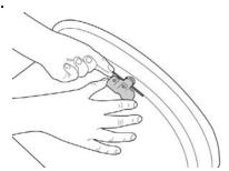
Place the anti-rotation pin into the valve hole to prevent movement of the sensor during tightening.
