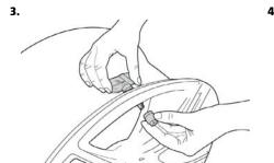
Screw the nut onto the sensor valve by hand.
