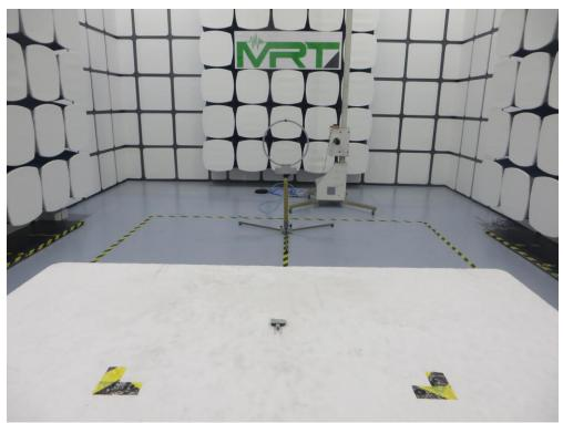
Test Mode: Mode 1 Description: Radiated Spurious Emission Test Setup (30MHz ~ 1GHz)
