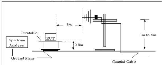
(C) Radiated Emission Test-Up Frequency Above 1GHz
