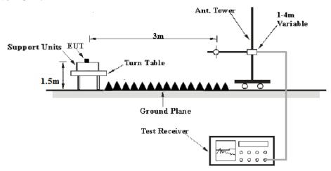
The radiated emission tests were performed in the 3 meters test site, using the setup accordance with the ANSI C63.10 - 2013. The specification used was the FCC  $\S$  15.209, 15.205 and 15.231.
