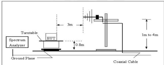
(C) Radiated Emission Test-Up Frequency Above 1GHz
