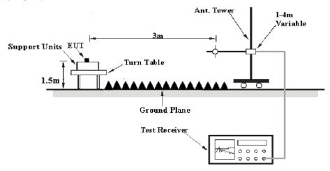
The radiated emission tests were performed in the 3 meters test site, using the setup accordance with the ANSI C63.10 - 2013. The specification used was the FCC part15.209, 15.205 and 15.231.
