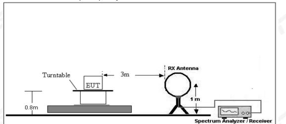
(B) Radiated Emission Test-Up Frequency 30MHz~1GHz
