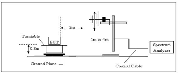
(C) Radiated Emission Test-Up Frequency Above 1GHz
