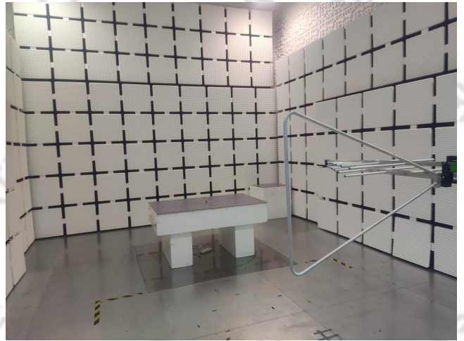
Radiated Emissions for 30MHz~1GHz
