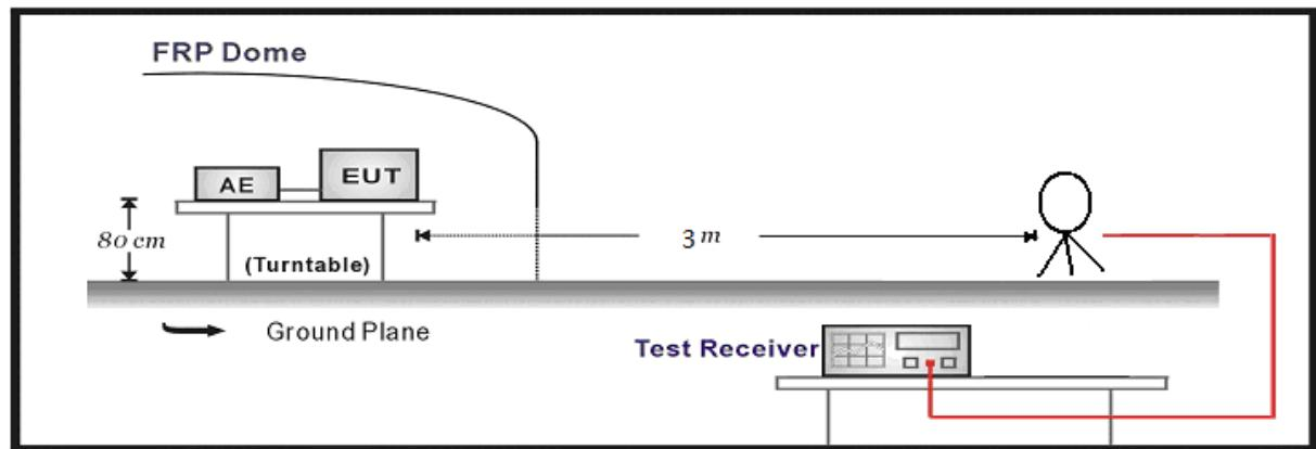
Below 1GHz Test Setup:
