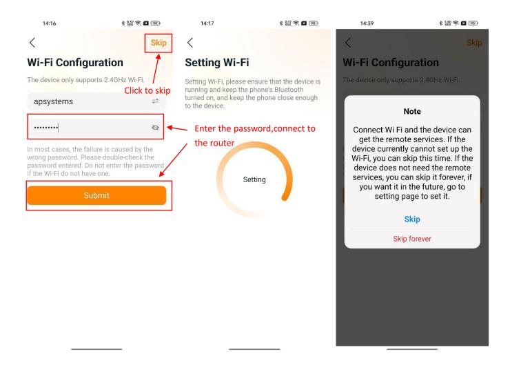
The remote service will not be available when the device is not connected to the Internet. You can use this APP to connect the APstorage PCS to the router via Lan or Wlan. (Please refer to chapter 4.5.3)
