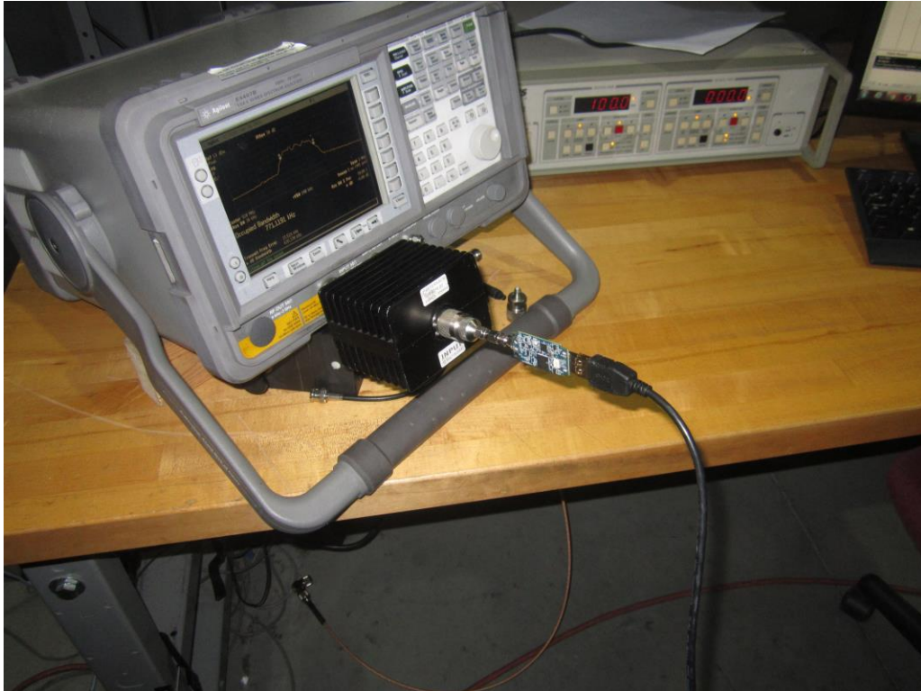
Conducted Emission at the Antenna Port (Close-up View)
