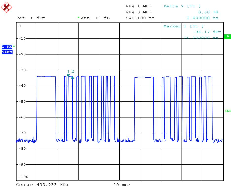
**1)Fundamental emission:****Antenna polarization: Horizontal:**
