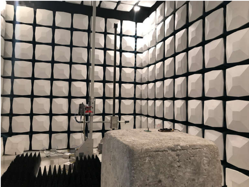
Description: Radiated Emission Test Setup for 1~18GHz
